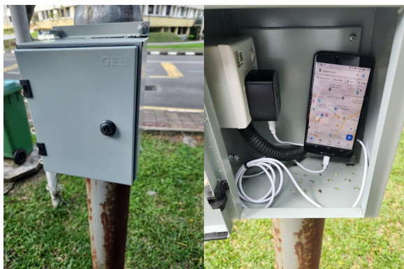
Figure 5 An Android IoT gateway is deployed inside a container box mounted on a bus stop pole in USM.
