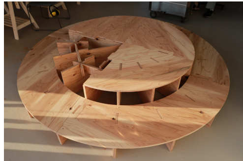
Figure 5: The completed stage, with one section of the floor removed.
