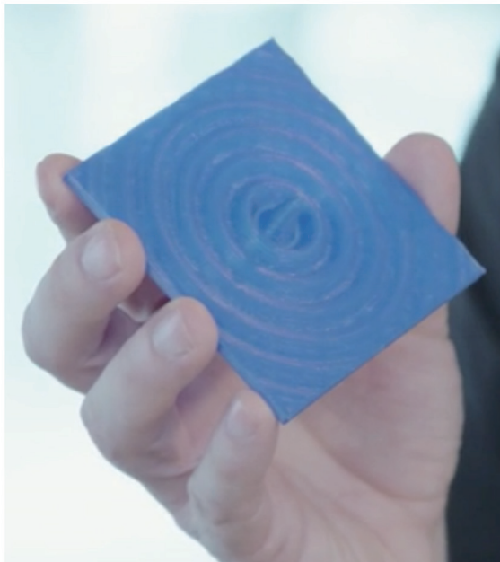
Figure 6: 3-D printed model showing propagation of a single wave from a point source.
