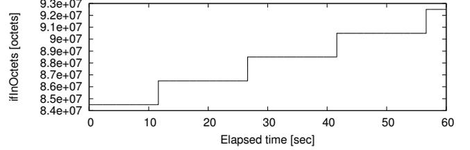
Fig. 19. Discrete nature of *ifInOctets* counter on a net-snmp agent
