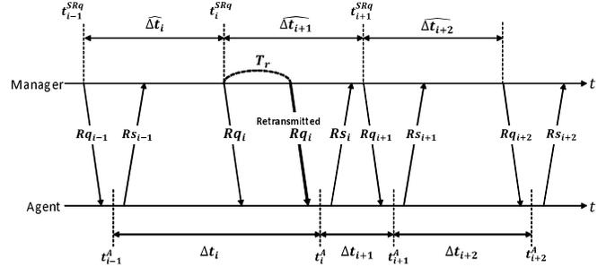
Fig. 7. Retransmission of a request
