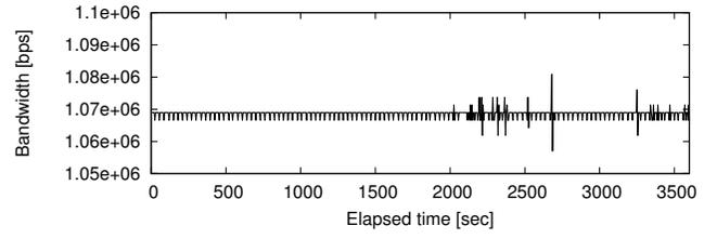
Fig. 14. Computed bandwidth utilization  $\widehat{Bw}_i$ : polling interval  $\widehat{\Delta t}_i$  is used as data interval  $\Delta t_i$
