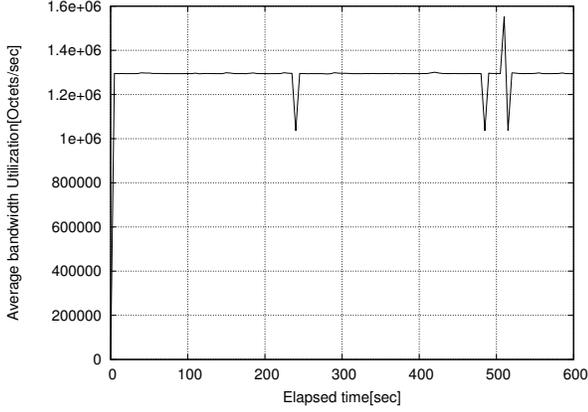
Fig. 21. Computed bandwidth utilization (Cisco Catalyst 3550)  $\Delta t = 5$  sec
