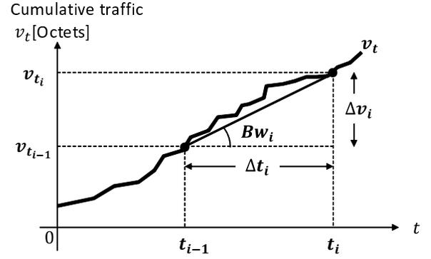
Fig. 2. Basic concept for calculating bandwidth utilization
