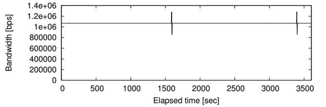
Fig. 8. Computed bandwidth utilization  $\widehat{Bw}_i$ : polling interval  $\widehat{\Delta t}_i$  is used as data interval  $\Delta t_i$
