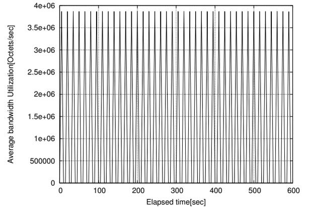
Fig. 20. Computed bandwidth utilization (Net-snmp)  $\Delta t = 5$  sec
