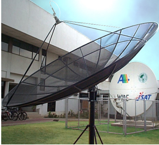
Fig. 3.1. AI 3 C band Receiving-Only and bidirectional antenna at AIT, Thailand
